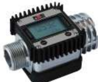
K24 F0040802A CAUDALIMETRO DIGITAL C/ TURBINA DIESEL 2 - 32 GPM PRESION 300 PSI 1" NPT
